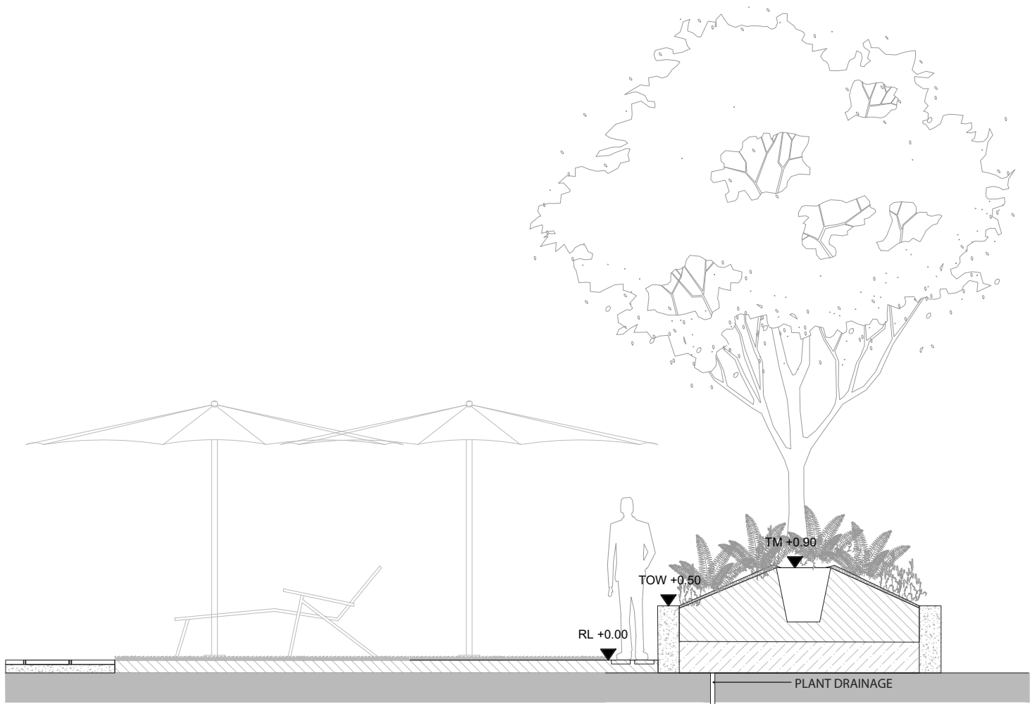
SECTION AA - GRASS AND RAISED GARDEN SCALE 1:50
